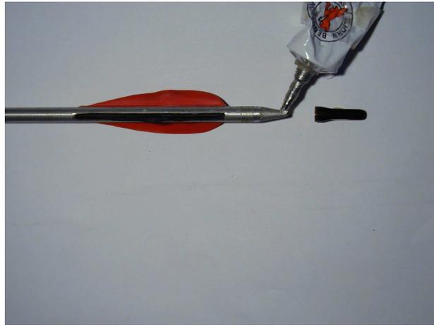
4. Present the nock on the shaft and rotate it for spreading the glue.
