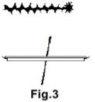
The arrow point is to the RIGHT in the picture and the nock is to the left end of the tear. The shaft is too weak. If the tear is 1 to 3 inches wide, the shaft can be stiffened by decreasing the weight in the point or decreasing bow strength. If the tear is greater than 3 inches, the shaft is too weak to compensate for. Select a stiffer shaft.
