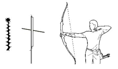
Verify your brace height, and then adjust the NOCK POINT until the tear is neither up nor down.
