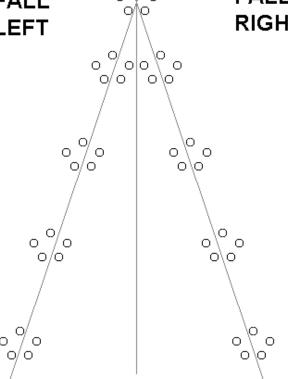
If the arrows fall to the left side of center, weaken the SPRING (CCW) until the arrows are in the center line.
