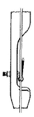
Adjust the PLUNGER until the left edge of tip of the arrow shaft is in line with the right side of the string. Do not use the left edge of the point of the arrow but rather use the left edge of the END of the shaft.
